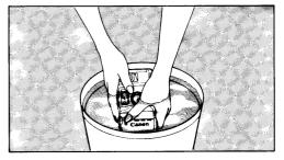
Before washing the camera, make sure that the back cover and the battery chamber are firmly closed.
